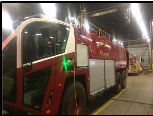
Photo 14 Crash 4, Model P-23, 420-gallon AFFF capacity.
