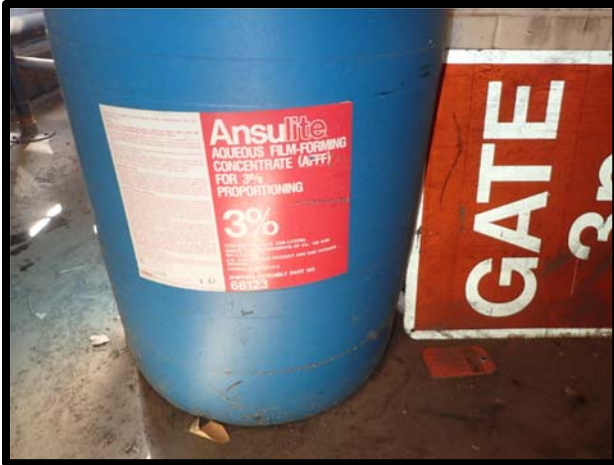
Photo 31 55 gallon drum of 3 percent AFFF found at Hangar 133 (Ansolite brand).
