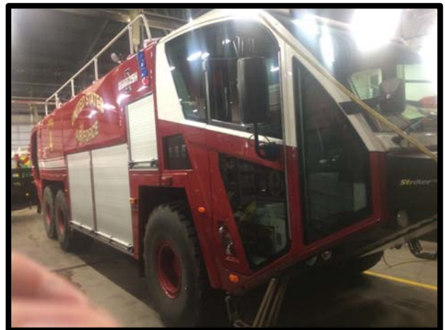
Photo 14 Crash 4, Model P-23, 420-gallon AFFF capacity.
