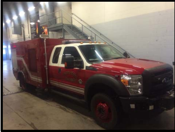
Photo 19 Rapid Intervention Vehicle, 56- gallon AFFF capacity.
