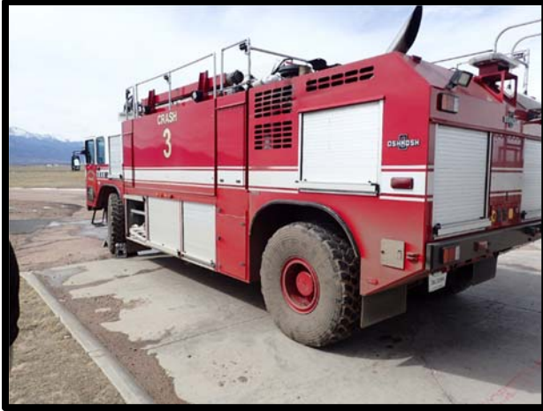
Photo 103 Crash 3, stationed at Fire Station #2, Model P-23, 210-gallon AFFF capacity.
