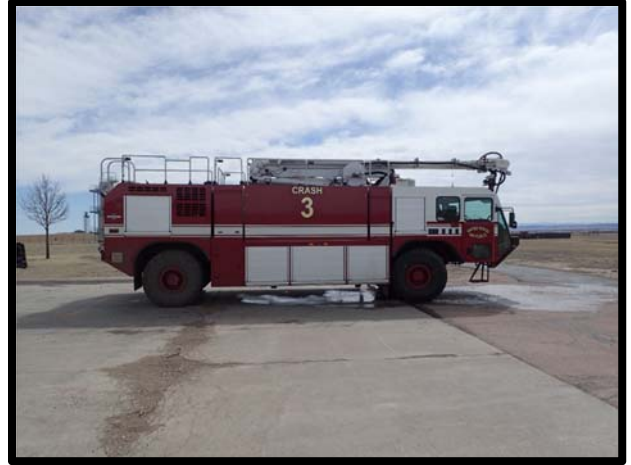
Photo 104 Crash 3, stationed at Fire Station #2, Model P-23, 210-gallon AFFF capacity.
