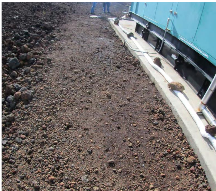
Photo 1: Jet A/Diesel impacted soil upon initial inspection. 2/1/23
